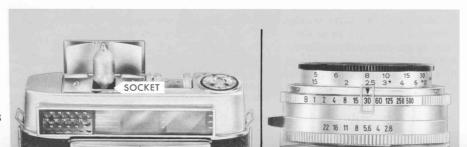
4. Lens Opening—From the Flash Guide Number table, opposite, select the proper flash guide number for the film you are using; divide this number by the camera-to-subject distance in feet (found in step 3) to find the nearest lens-opening number. Rotate the lens-opening scale by its black handles until this number is opposite the index mark. For example, if KODACHROME-X Film were loaded in the camera,
