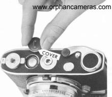
Battery—The life of the battery, supplied, is approximately two years.\* To replace the battery, turn the coin-slotted battery COVER counterclockwise, move the milled lever aside, and remove the cover. Remove the used battery and replace it with a PX-13 type mercury battery, inserted with its positive side (+) toward the inside. Replace and fasten the cover by turning it clockwise. \*With average use.
